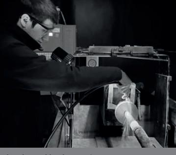
MPI station equipped with Johnson & Allen bench, capable of processing parts up to 2,5 meters in length. FPI station equipped with custom penetrant system line. Magnaflux chemicals. Olympus Nortec & Epoch flaw detectors. Wide range of reference standards and probes. Customized NDT solutions.
